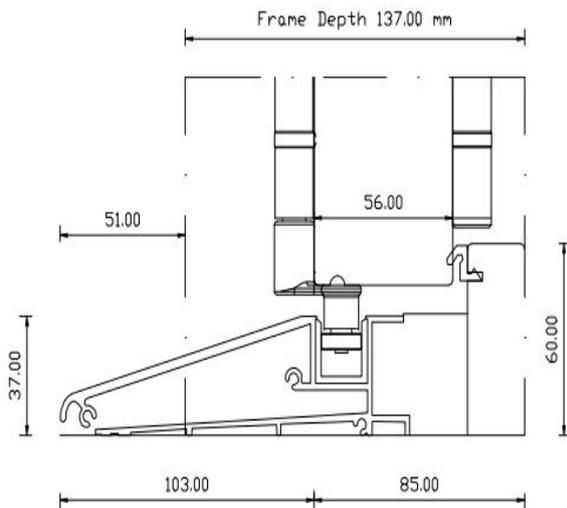
We always recommend aluminium cill instead of timber cill with aluminium track, as it's more durable, resistant to wear and tear damage and keeps its original look for years after installation.
